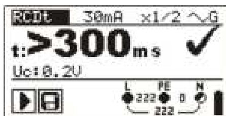
Figure 5.19: Example of trip-out time measurement results
