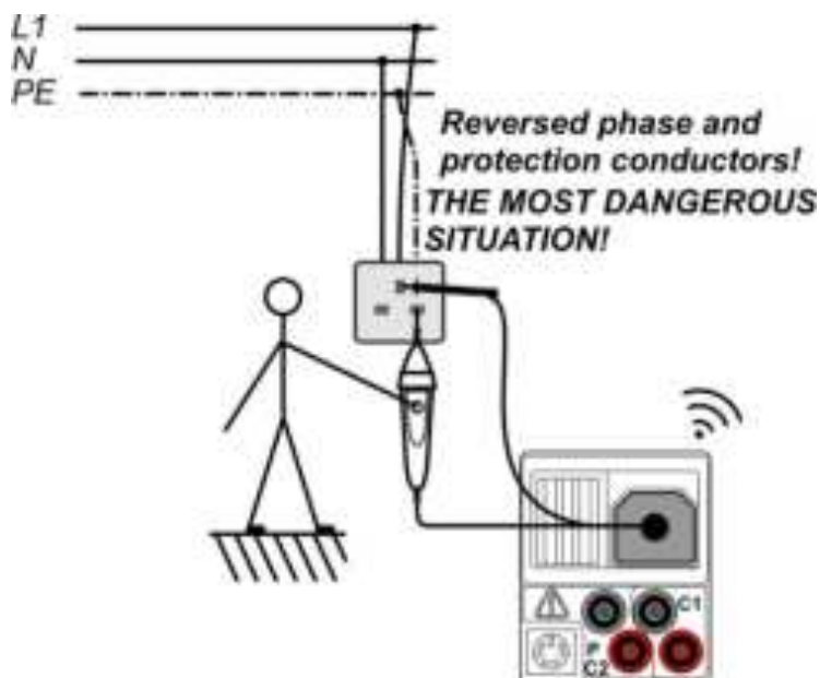
Figure C.3: Reversed L and PE conductors (application of tip commander)
