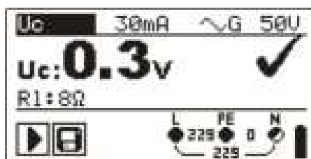
Figure 5.18: Example of contact voltage measurement results
