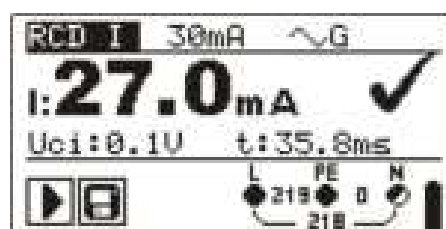
After the RCD is turned on again
