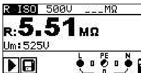
Figure 5.10: Example of insulation resistance measurement result
